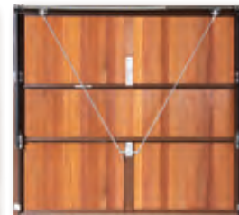
Both retractable and canopy doors have twin latches operated by rods or cables from a locking handle. Two at the bottom for retractable doors, two at the top for canopy doors.
