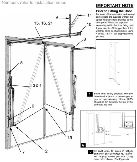
Swing the pivot arms up, align two holes in each lower side seal with those in main pivot brackets. Ensure lip on lower side seal locates against side of jamb for full length of side seal. NOTE: for special sized doors the bottom of side seal must be cut short to suit installation.
