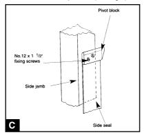
Smooth lower side seals into position. Align pivot blocks with holes in lower side seals as shown. (Fig. C) drill pilot holes and secure using two no.12 x 1<sup>1</sup>/2": self tapping screws per block.
