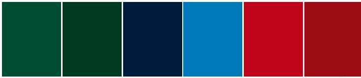
Moss Green RAL 6005 Fir Green RAL 6009 Steel Blue RAL 5011 Light Blue RAL 5015 Flame Red RAL 3000 Red RAL 3003
